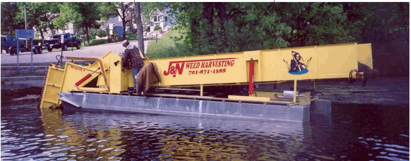
A mechanical harvester could be used to create cruising lanes through several areas of dense growth in VanVliet Lake.
